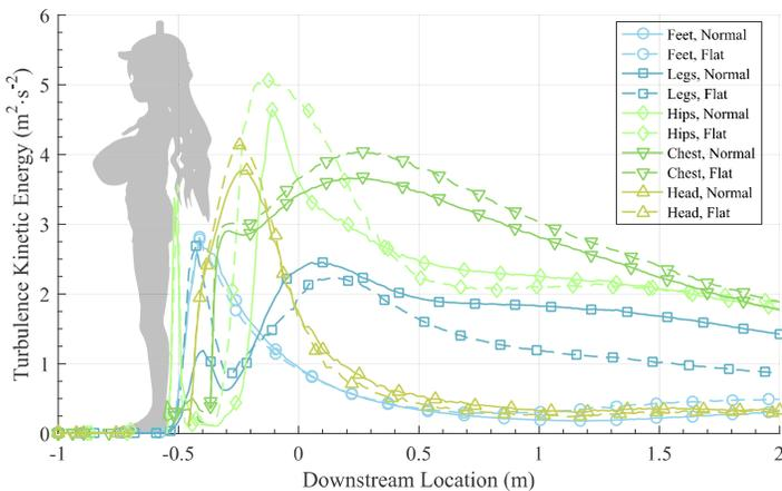
**Figure 17.** Comparison of TKE at 5 z-locations centered along  $x = 0$  and ranging from  $-1 \leq y \leq 2$  meters. Lucoa positioned and to scale with x-axis. Feet  $z = 0.1\text{m}$ , Legs  $z = 0.5\text{m}$ , Hips  $z = 0.9\text{m}$ , Chest  $z = 1.18\text{m}$ , Head  $z = 1.55\text{m}$ .
